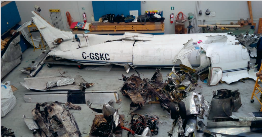
Remains of Carson Air Metro II freighter were gathered inside TSB laboratory for detailed analysis
